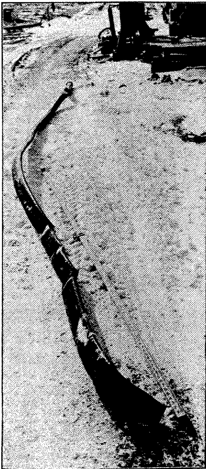
4½" TUBING FROM SALT WELL ILLUSTRATING FORCE OF FALLING CAVITY DEBRIS AND ROOF ROCK. TUBING WAS PULLED THROUGH 8 5/8" CASING.
